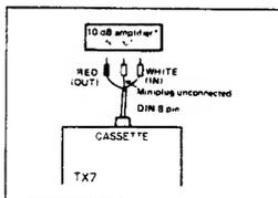
\*Use an 10 dB amplifier or set a cassette deck to REC/PAUSE and adjust it so that there is 10 dB gain.
