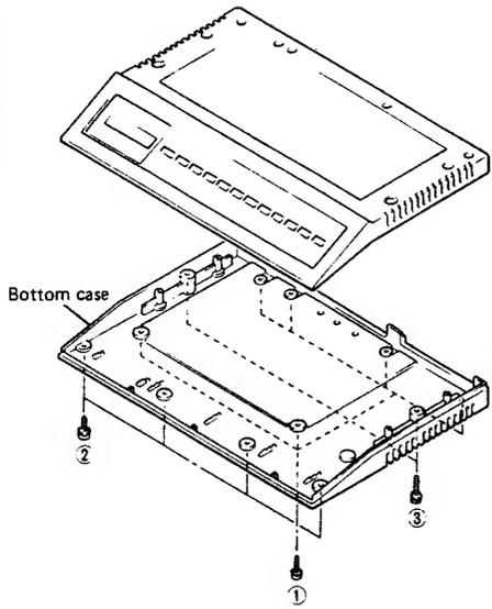
1. Removing the Bottom case
