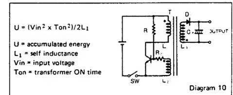
The operation of the RCC circuit is as follows.
